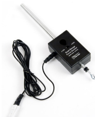
Hook for connecting to a string and measuring pulling force
