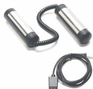
The Hand-Grip Heart Rate Monitor measures a person's heart rate by registering the small electrical signals carried across the surface of a person's skin each time his or her heart contracts. This signal is measured at the surface of the skin by electrodes embedded in the hand grips of the Hand-Grip Heart Rate Monitor. By graphing this signal, the heart rate can be determined. A sample graph is shown below.
