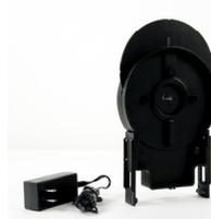
The plane of the luminous sources is located at the position marked by the pointer on the base. In contrast, the LED point source is located at the back edge of the holder. This location is important to note for accurate distances in inverse-square experiments.
