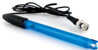
The Vernier Gel-Filled Combination pH Electrode is designed to be used with the Vernier Electrode Amplifier (order code EA-BTA) to make measurements in the pH range of 0 to 14. Our pH Electrode can be used for any lab or demonstration that can be done with a traditional pH meter, including acid-base titrations, monitoring pH in an aquarium, and investigating the water quality of streams and lakes.
