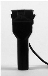
*Push in the two latches at the top of the handle so that they splay outward*
