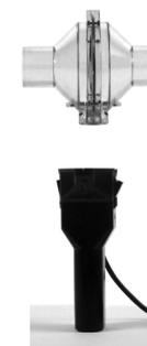
*Pull up on the Flow Head and remove it from the handle.*
