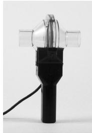
*Press down firmly on the Flow Head until it securely attaches to the handle. Push the latches in to lock the Flow Head in place*
